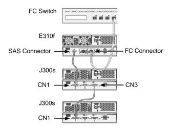
You can expand a SAN system with no single point of failure. See Figure 14. Such an arrangement requires:
